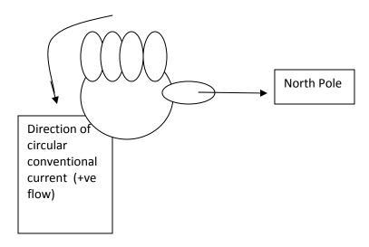
Remember: It's conventional flow again! We are interested in the direction of +ve flow (not electron, -ve flow)
